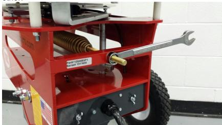
**Step 13** – The pull cord or optional radio release can now be connected to the machine. The manual or optional wireless release connects to the yellow-ended wire plug.
