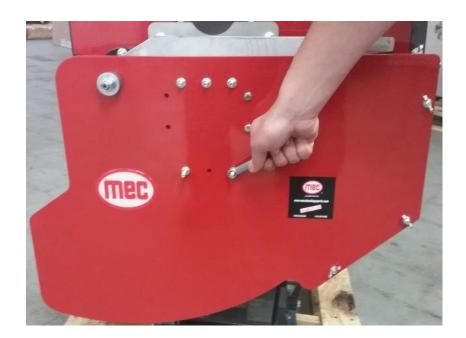
**Step 6 -** Un-wind the two locknuts enough so that when a Rabbit clay is loaded the deflector supports it and holds the clay against the throwing plate as shown below.
