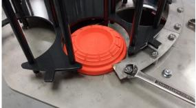
**Step 4** – Put some clay's in the carousel, but do not fill just yet, as this will make it easier to adjust the elevation and tilt of the machine. It should be pointed out that if the machine is tilted forward, it will throw a low target along the ground. Tilting all the way back will allow the machine to throw a vertical teal target.
