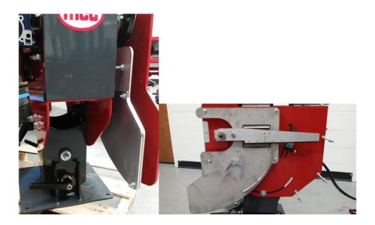
**Step 3** – With the Rabbit Plate removed, it now needs to be attached to the front side of the Throwing Plate as shown in the photo below. Simply hold the plate straight to the throwing plate and push the front rail to the full open position. Slide plate on and release the front. Replace the Allen bolts to securely attach the rabbit plate to the throwing plate.
