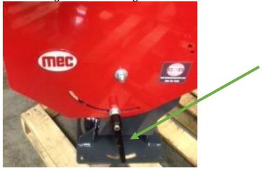
**Step 6** – Adjust machine tilt by loosening the black lever at the front of the square base plate upright slot. The machine can be tilted to one side to allow the target to curl. When viewed from behind, the machine can be leaned further to the left for a dome down type target when throwing standard clays only.
